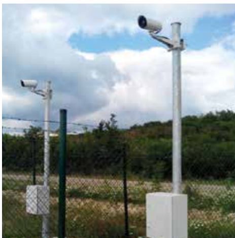
Thermal imaging cameras need no lighting equipment whatsoever and will operate with the same accuracy during night and day.
