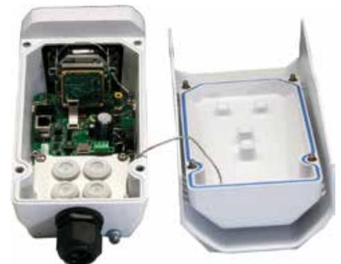
FC-Series S is intended for outdoor applications and has protection circuitry that only allows the intended signaling to pass through.
