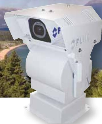
A FLIR FC-309 is mounted on a Pan-Tilt-Zoom (PTZ) system that allows for 360° continuous rotation.
