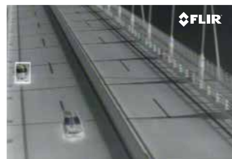
Stopped vehicle detection
