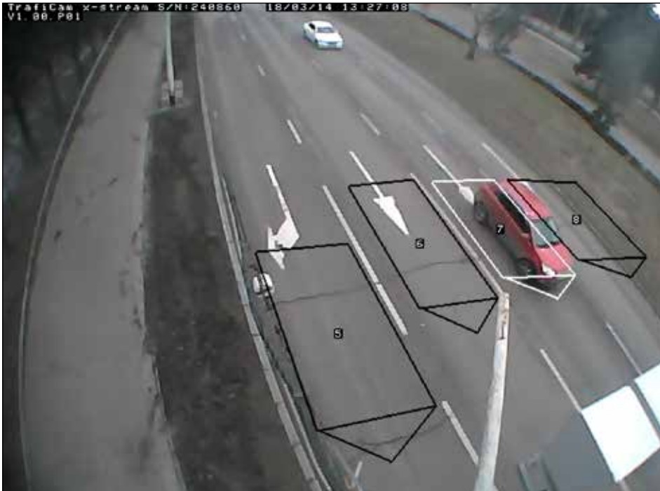
TrafiCam x-stream is an IP-addressable device that provides MPEG-4 or H.264 color streaming video at full frame rate to the control center for general intersection surveillance.
