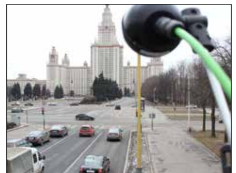
The Traficam x-stream vehicle presence sensor combines a CMOS camera and video detector in one single unit.
