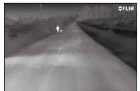
Thermal imaging night vision systems onboard trams allow drivers to see clearly in total darkness.
