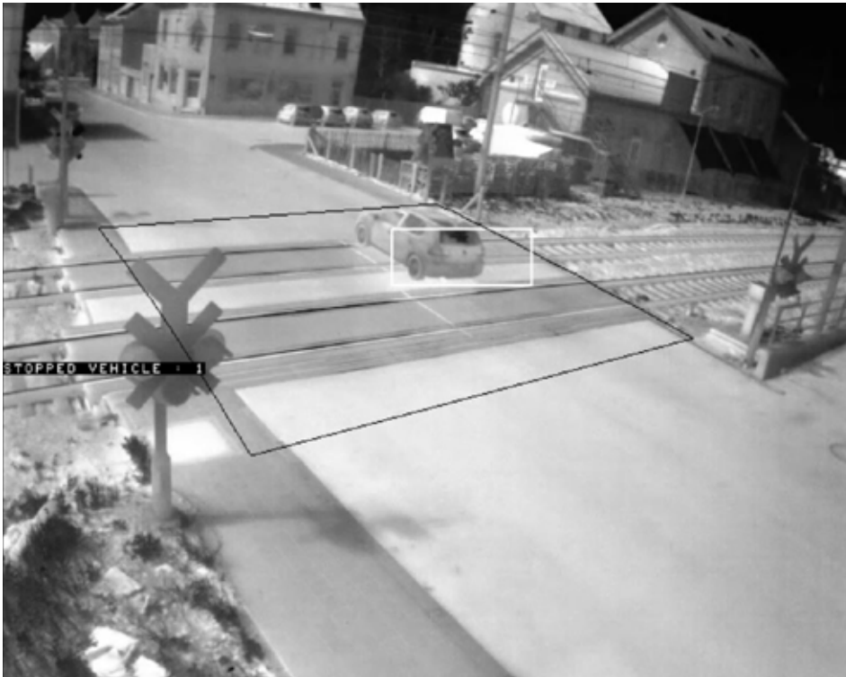
Vehicle detection at a level crossing
