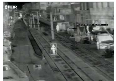
Thermal imaging cameras can detect people walking on the tracks and trigger a message on a VMS panel in order to alert the tram driver of a potential dangerous situation
