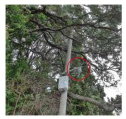
ThermiCam can distinct between vehicles and bicycles based on heat information coming off these road users and will transmit its detection information over contact closures or over IP to the traffic light controller.
