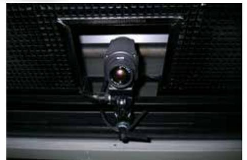
A central solution: TOPA installed a FLIR A310 with 45° wide-angle lenses in each of 10 dynamometers.
