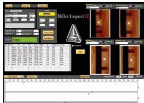
Test screen with corner defects on a square billet as detected by an InspectIR system with four thermal imaging cameras
