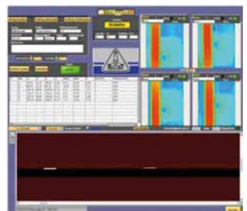
Test screen with corner defects on a square billet as detected by an InspectIR system with four thermal imaging cameras
