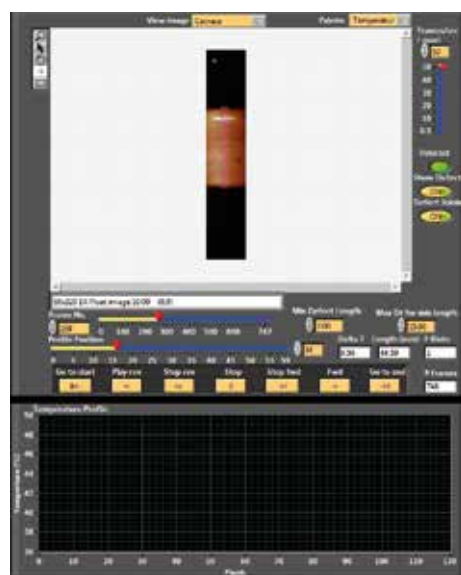
This InspectIR screenshot shows a steel bar before analysis. In the top view, there's a thermal image of a bar or billet, with everything but the area of interest filtered out. The white line on the steel bar indicates a surface breaking defect.
