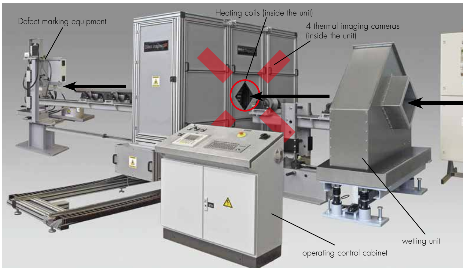
The billet InspectIR consists of a thermal imaging camera enclosure, signal processing system, operating control cabinet, induction heater, induction coils, water cooling system, conveyor and defect marking equipment.
