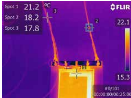
Cables with a low current rating are put to the test. If approved for use, these cables will contribute to keeping the weight of the car low.
