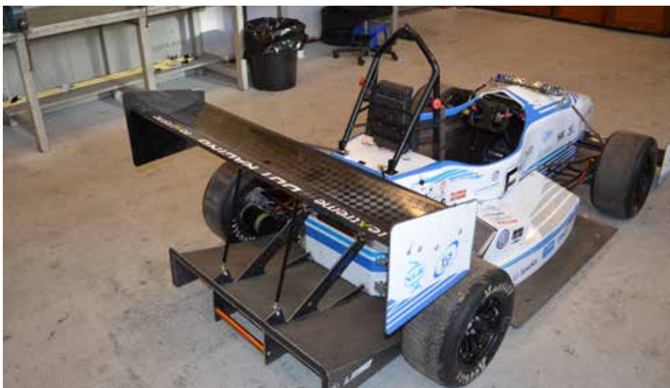
The current DUT car weighs 175 kg, whereas many competing teams are struggling to build cars even below 200 kg.
